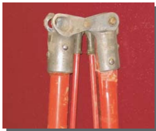
Broken Pole Stock
