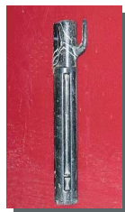
Cracked Ferrule Head
