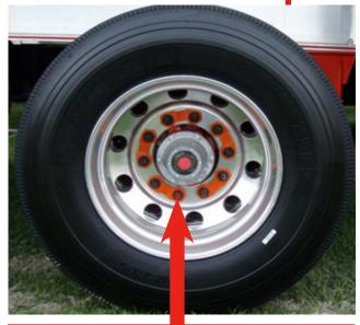
Lug nuts can be re-torqued without removing the Zafety Lug Lock<sup>®</sup>
