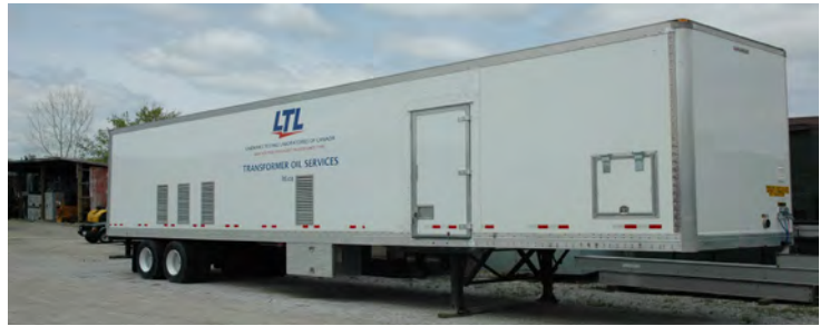
State-of-the-Art Mobile Oil Regeneration Plant
