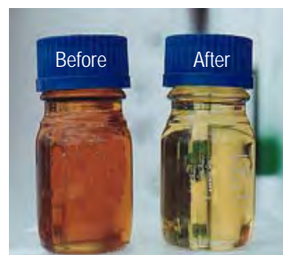
Tx Oil Before and After Regeneration
